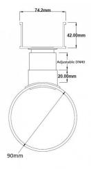
Grates longer than 1500mm supplied in sections. Tile Inserts longer than 1200mm supplied in sections. Channels over 3000mm supplied in sections with joiner. +/-2mm tolerance on dimensions
