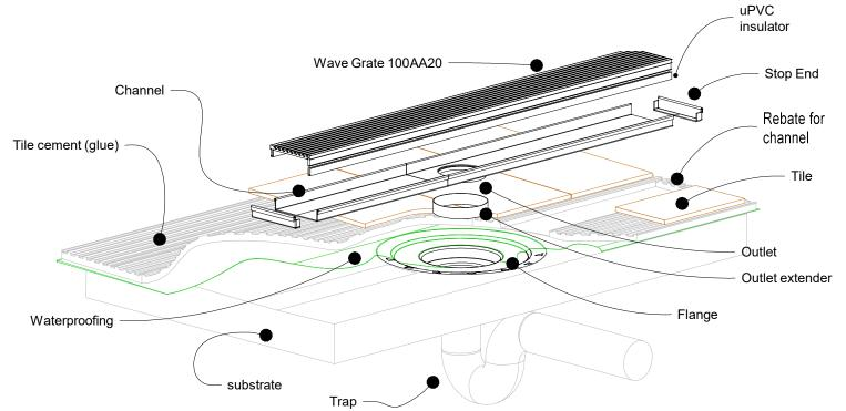
NOTE, this method requires the channel system to be ABOVE and SEPARATE from the WATERPROOFING.
